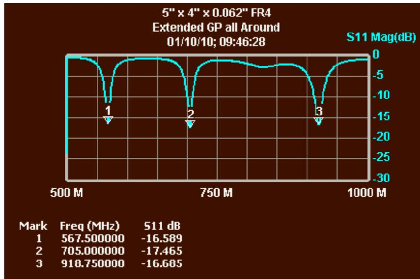
Figure 4—Extended Ground Plane on All Sides
