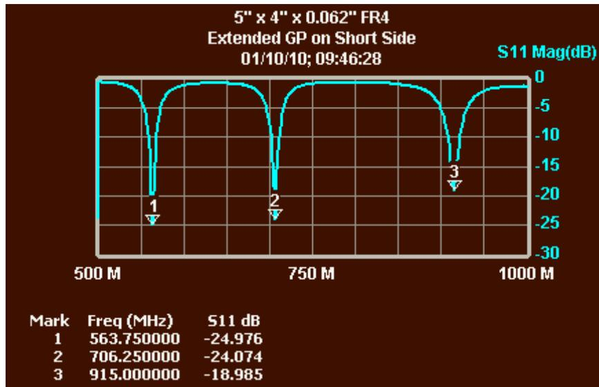
Figure 3—Extended Ground Plane on Short Side
