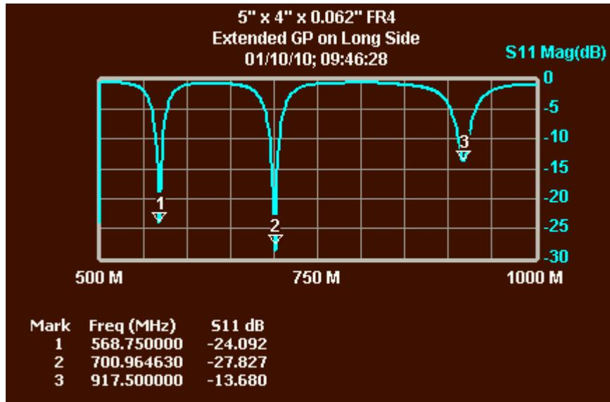
Figure 2—Extended Ground Plane on Long Side
