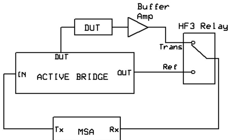
**Figure 2—Transmission/Reflection Test Set for MSA**
