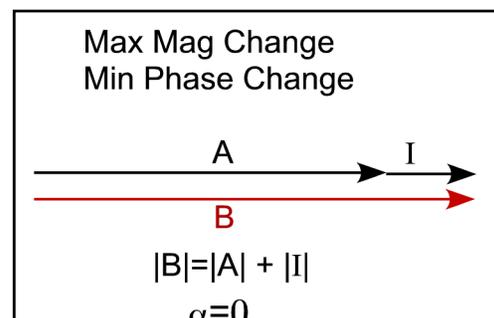
**Figure 1—Vector diagrams of combined signals A and I, producing B.
